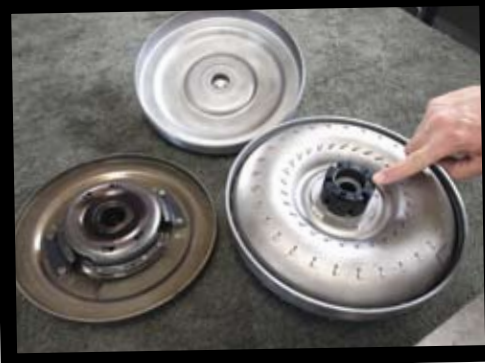
Carr is not a proponent of lockup torque converters in high-performance applications. He says OE lockup clutches lack enough surface area to harness real horsepower, aren't worth the weight penalty, and sap power and dull throttle response due to the added mass. The finger points to the machined composite spacer that's installed inside CPT's 12-inch nonlockup converter in place of the clutch assembly ( on left ) that weighs 9 freakin' pounds. This CPT 12-inch converter has a 2,200-stall speed and is intended for use in 450hp street machines.
