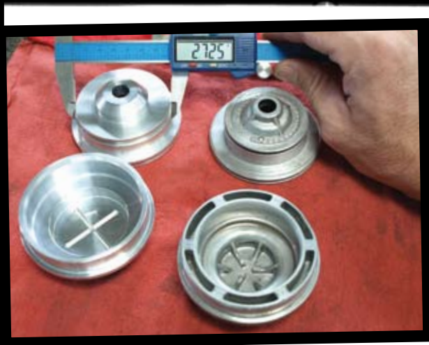
The 2.350 diameter of the stock Second gear apply servo ( right ) limits its ability to apply pressure on the Second gear band. Carr solves the matter with his billet aluminum Super Servo (PN 12279). At 2.725 inches, it has more surface area than even the scarce Buick Grand National unit. The Super Servo holds the Second gear band with more clamping force to increase life while delivering crisper 1-2 upshifts.
