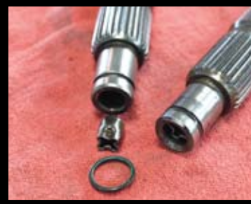
Getting back inside the transmission, when a 200-4R is used with a non-lockup converter, the check valve and seal located in the end of the input shaft must be removed ( left ). These parts apply the lockup clutch feature in a stock transmission but are unnecessary. A fringe benefit is there's now more fluid available to lubricate the planetary gearset. A stock lockup-style input shaft is shown on the right for contrast.
