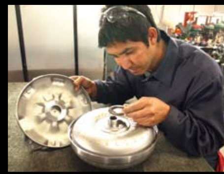
CPT also offers 9- and 10-inch nonlockup torque converters for the 200-4R. Here, converter assembler Juan Jimenez gets one ready for final assembly. In the case of CPT's 10-incher, careful selection of internal parts—particularly the stator—results in a torque converter that can handle 800 hp, stalls at 2,800 rpm, yet still delivers efficient highway cruising at 1,800 rpm. It's a favorite with Carr's Chevy 502 and 572 customers. The all-out 9-inch converter offering stalls at 3,500 to 3,800 rpm, but its stator design is efficient enough to cruise at much lower rpm in Overdrive.
