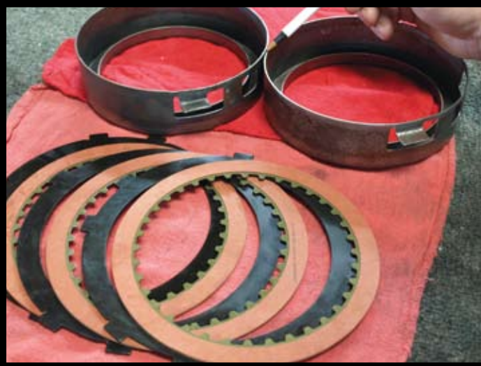
The stock overdrive clutch assembly uses three steels and two clutch plates. By removing 0.080 from the overdrive apply piston ( pen points ), Carr can add a third clutch plate for a 33 percent increase in torque capacity. Unlike a 700-R4, the 200-4R is not prevented by its valvebody program from running in Overdrive at wide-open throttle. The extra clutch capacity assures your 502 Rat motor won't overpower the clutch in triple-digit Cannonball Run mode.
