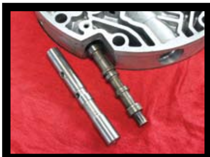
On the stator side of the oil pump, the stock lockup valve ( right ) is replaced by a machined steel valve ( left ) that redirects the hydraulic circuitry to suit the conventional (nonlockup) torque converter.
